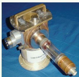
3 MW S-band (2.998 GHz) tunable pulse magnetron
