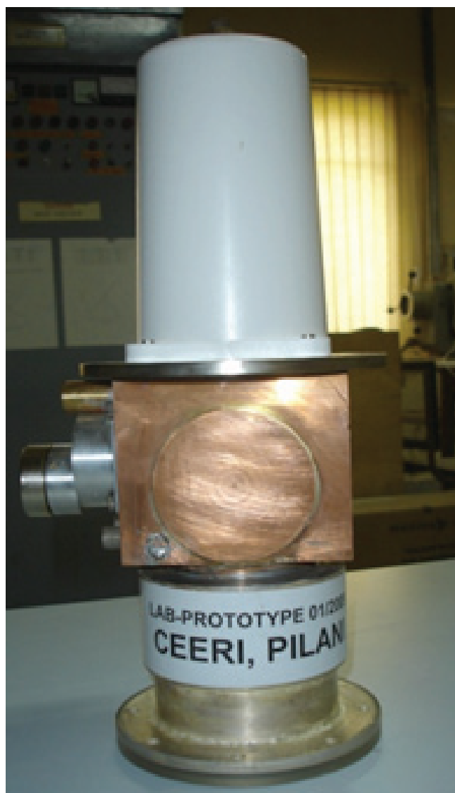
2.6 MW magnetron at it testing in LINAC System
