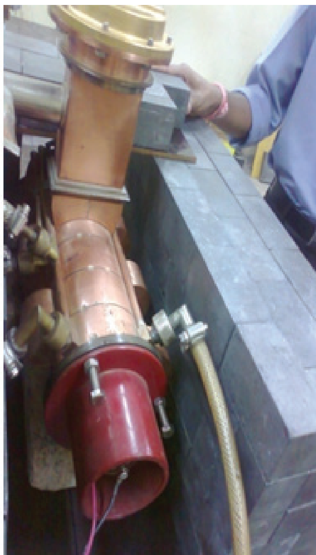
2.6 MW magnetron at it testing in LINAC System
