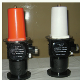
2 MW S-band tunable pulse magnetron
